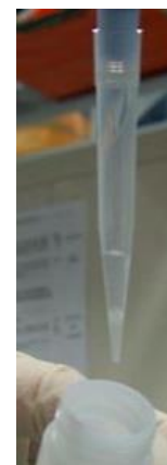
Fig. 2: recommended volume of beads per Lysis buffer in the pipette tip
