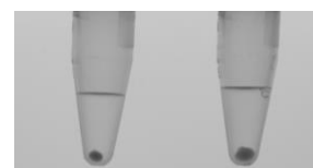
Fig. 1: recommended pellet sizes: Left: max. pellet bacterial size Right: max. pellet size for particle containing samples
