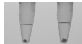
Left: max. pellet bacterial size Right: max. pellet size for samples containing yeast or particles
