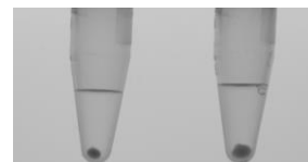
Fig. 1: recommended pellet sizes: Left: max. pellet bacterial size Right: max. pellet size for particle containing samples
